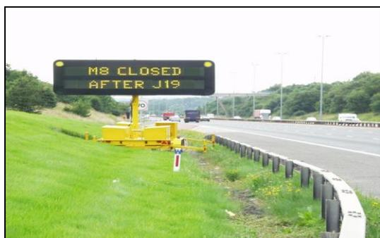
**Figure 7 – Example of a Mobile VMS Displaying Network Information Message**
